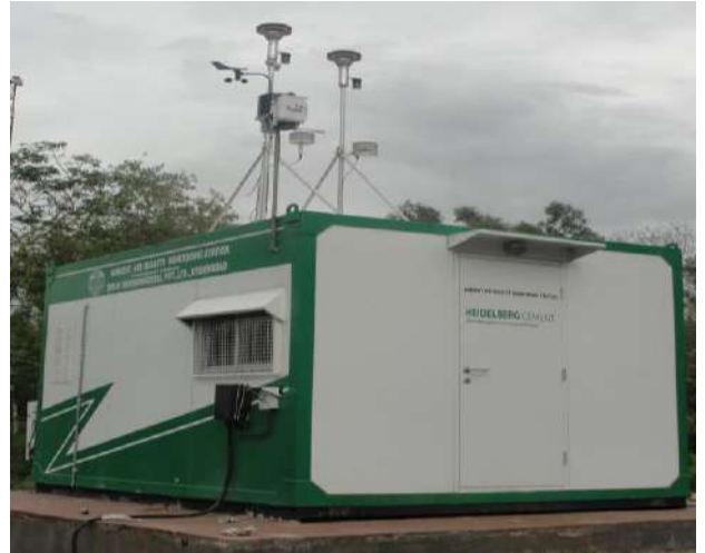
Continuous Ambient Air Quality Monitoring stations at HCIL, Narsingarh (02 Nos Locations)
